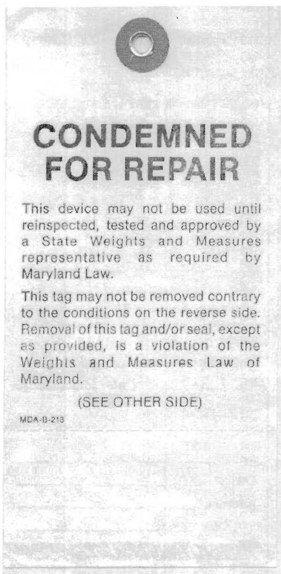
Condemnation tag indicating the scale or pump has failed inspection and repair must be undertaken before scale can be put back into use.
